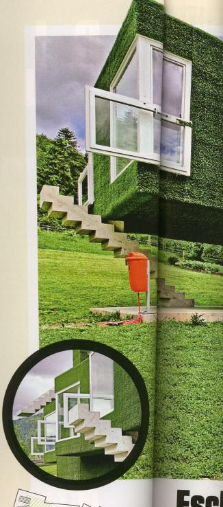
Depending on its position, each cast-concrete staircase can be a support pillar, be simply decorative, or provide access to an exterior level
